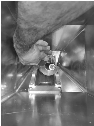
Fig. 39 - Spiral removal
