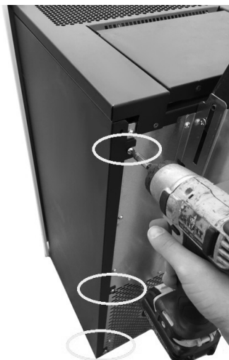
Fig. 26 - Loosen screws
