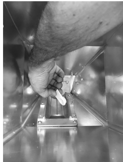
Fig. 40 - Bearing removal
